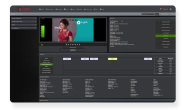
A key feature of the Cubix Content Discovery engine is the efficient use of bandwidth when uploading to the cloud. By sending full frame still images (uploaded at pre-configured intervals), whole 'chunks' of video no longer need to be uploaded with the associated increase in transport and storage costs. Cubix will then automatically combine this resulting metadata with the asset.
